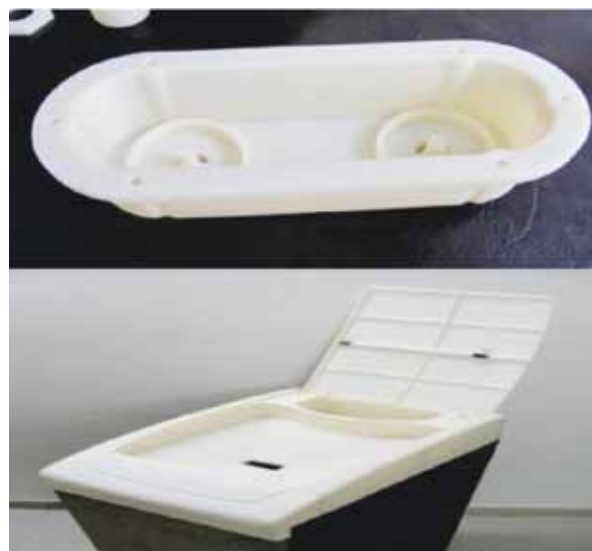
Manufactured at IGTR, Ahmedabad through FDM technology
