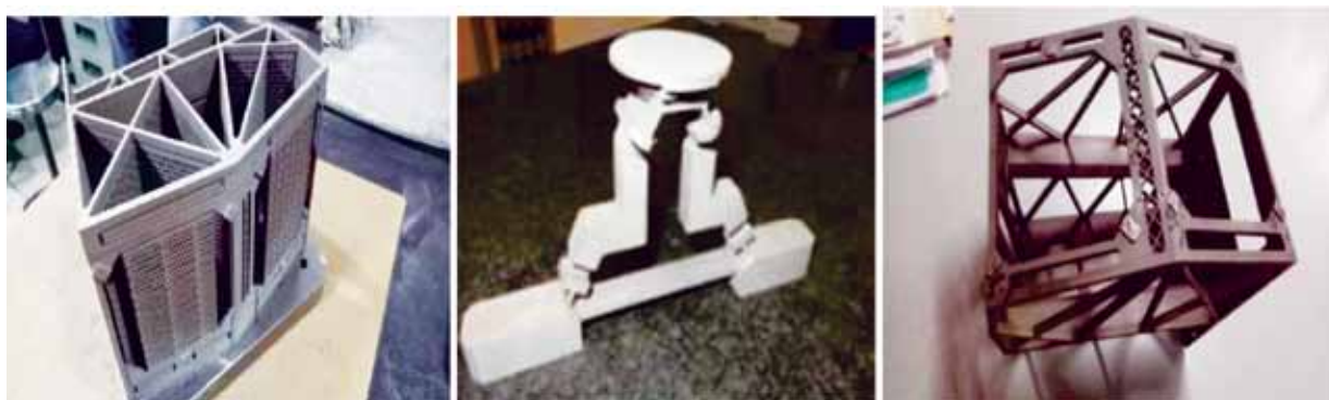
Some complex products developed through Metal RPT by IGTR, Ahmedabad
