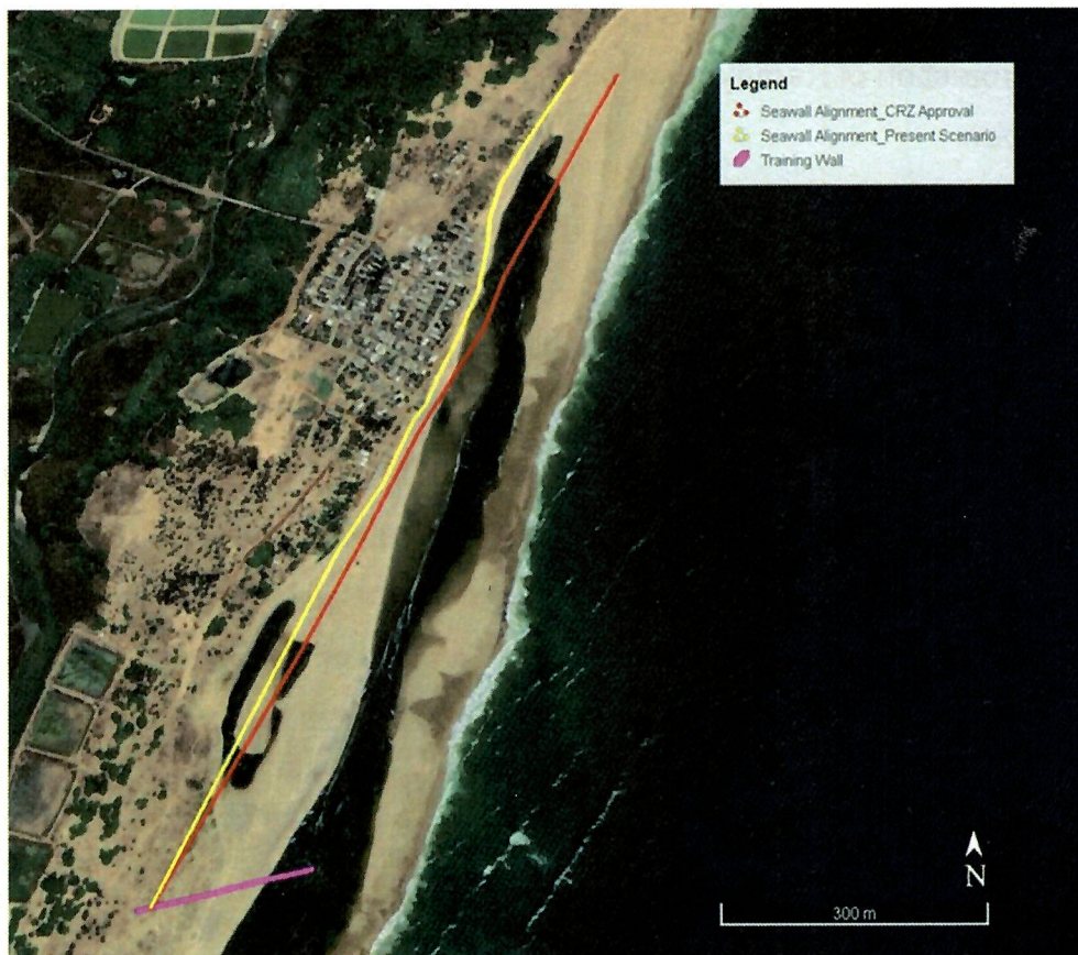
Figure 1: Alignments of CRZ approved seawall(red), seawall as per the present shoreline(yellow), and training wall
